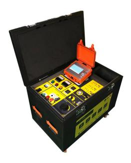
GD-4138 Cable Fault Locating System is important tool to maintain all kinds of cables. It is compatible equipment that can trace, locate the underground cables, with fault distance measurement and HV generation. As it is movable device, it is convenient to carry on-site. If acoustic locator is used together, it can locate accurate position of cable fault point. Application is underground cable, aerial cable, power cable, local cable, communication cable and fiber cable.
